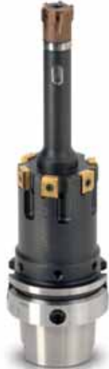
DIHART® special tool 2-stage reamer on HSK 63 1st stage modular and adjustable TiN-coated for Ø 20 H7, 2nd stage fixed and modular, DBF-coated for Ø 50H7.
