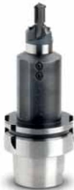
JEL® special tool VABOS-K with thread milling cutter M14x1.25, with PCD. Three operations with only one tool – for pre-cast rough drilling to core bore dimension, production of 90° and face counterboring Ø 22 mm, thread milling M14x1.25.
